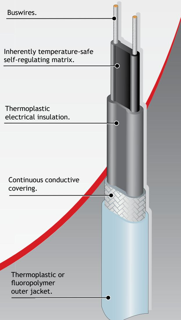
*FLVw-CF is supplied with a black fluoropolymer outer-jacket.*
