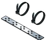
Stainless steel fixing bracket complete with 2 x nylon tie wraps, with several functions. Used in wide gutters to provide equal spacing for double runs of GT heating cable. Also used to protect heating cable in difficult transition zones and supporting heating cable in drainpipes.
