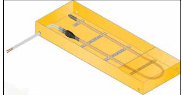
Points System Drainage Tray Heater
