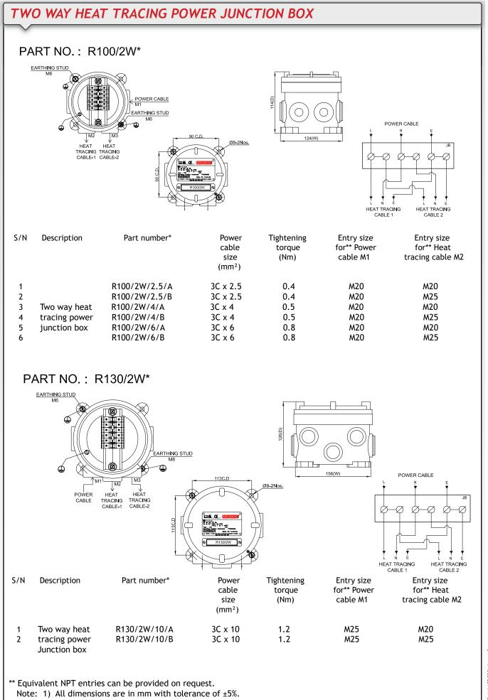
2) External earthing stud is fitted with PVC sleeved copper lug.
